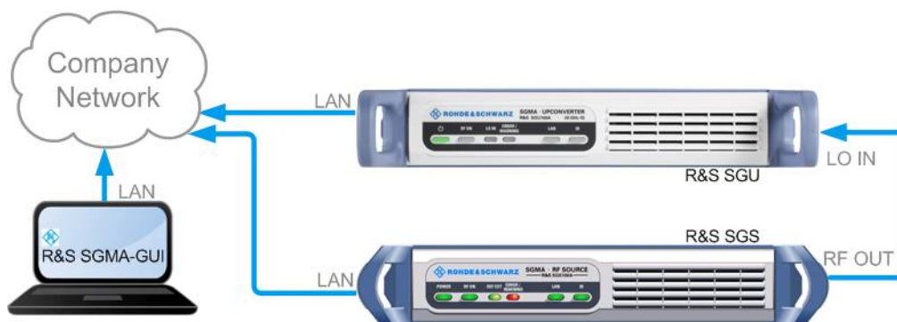
Figure 5-5: Connection of an R&S SGS and an R&S SGU in a company network
