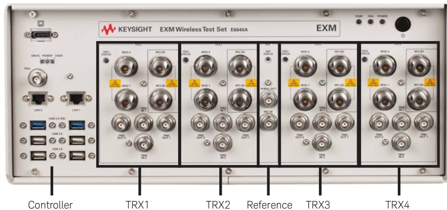
Figure 2. EXM's system hardware architecture (4 TRX configuration)
