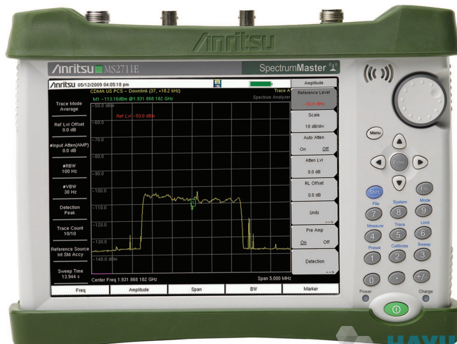
Spectrum Master™ MS2711E Spectrum Analyzer featuring 8.4 inch Daylight Viewable Touchscreen Compact Size: 273 mm x 199 mm x 91 mm (10.7 in x 7.8 in x 3.6 in), Lightweight: 3.45 kg (7.6 lb)
