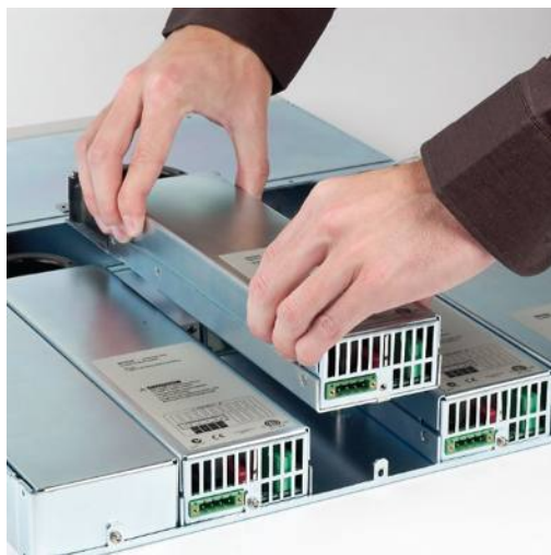
Figure 6c. User re-configurable modular system
